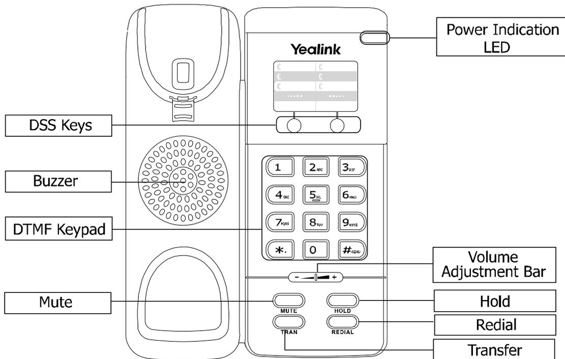
You can check the following list which introduces the IP phone's keypad in details:
